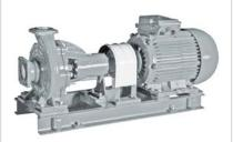
Intended for pumping of water with temperature up to 105 °C, solids content below 0.1% by mass, solids size below 0.2 mm
