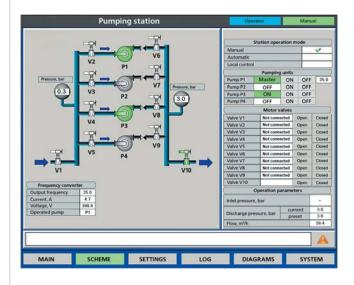
Intended for a complex automation of the water supply facilities: borehole water intakes, water storage tanks, 2-nd & 3-rd lift pumping stations, measuring points, booster stations, auxiliary process equipment
