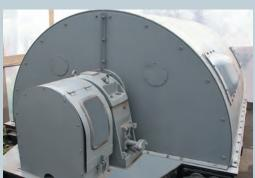
The electric motors are intended for driving the water injection pumps and auxiliary machinery at Rumaila oilfield cluster pump station (CPS).
