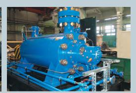
The water injection pumps for the cluster pump station (CPS) are intended for formation pressure retention at the Rumaila oil and gas field in the south of Iraq.
