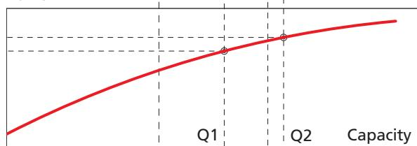
Fig. 9. Pump operation with excessive head
