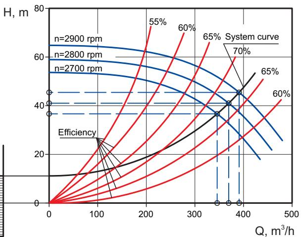
Fig. 7. Pump operation in system with predominant friction losses in case of speed control
