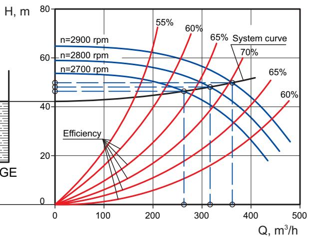
Fig. 8 Pump operation in system with predominant static part in case of speed control
