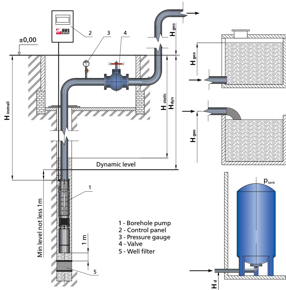
Fig. 3. Typical water intake options
