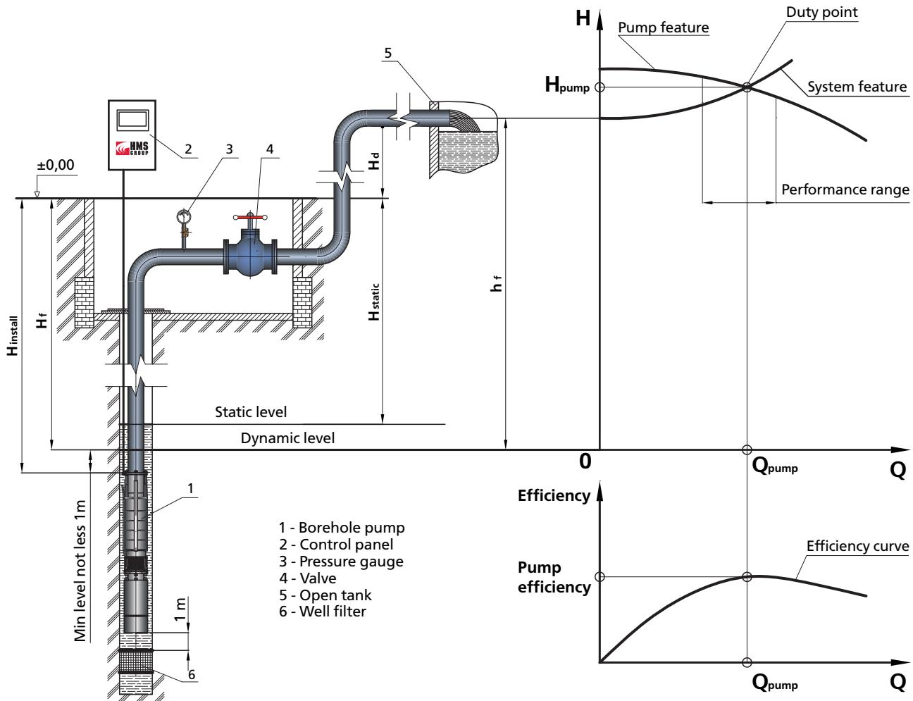
Fig. 2. The pump and the water supply system installation features
