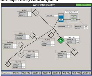
Intended for complex supervisory control of water supply and sewage disposal facilities with automatic or supervisory control (including remote) of the process equipment
