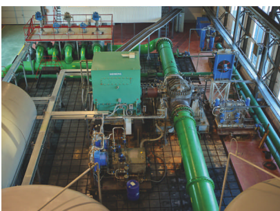
Figure 4. The stand is a full-scale OPS model and provides comprehensive testing of all unit components and systems in all modes.
